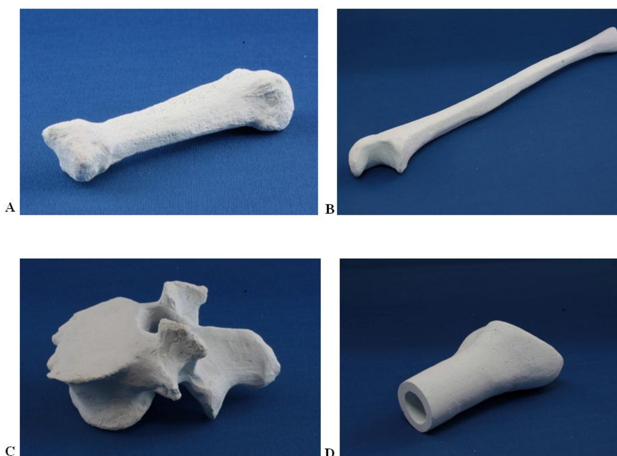
Fig. 1: Custom made constructs made of biphasic calcium phosphate ceramics. A – phalanx, B – ulna, C – vertebra, D – section of a tibia showing the space corresponding to the medullar zone.
